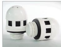
**Vent Plugs** – Specially designed incorporating a microporous ceramic filter which effectively returns all acid spray to the cell, but allows free exit of oxygen and hydrogen which is generated towards the end of boost charging.
